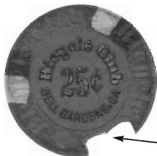
Material Removed for the Edge Insert
